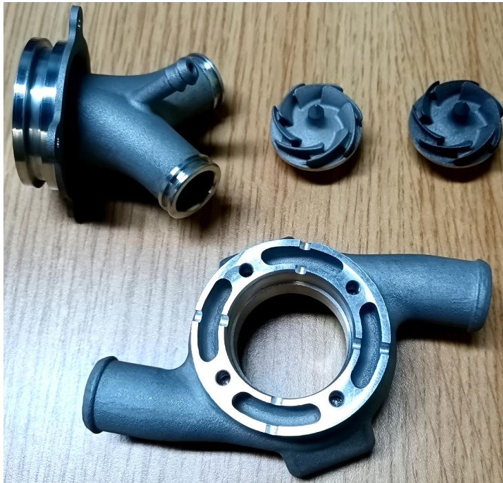
Aluminum 3D printed with CNC processed parts for automotive industry
